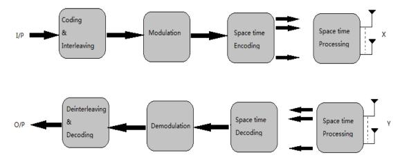
Figure 4. MIMO System Block diagram
