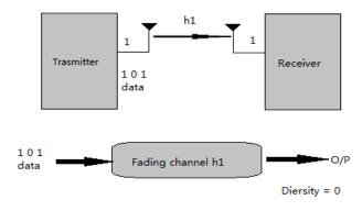
Figure 2. Zero Diversity between transceiver pair
