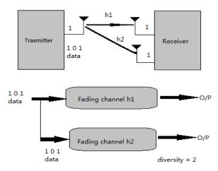
Figure 3. With Diversity between transceiver pair
