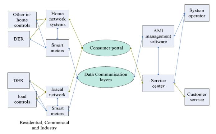
Figure 1. Composition of an AMI system (Sui et al., 2011)
