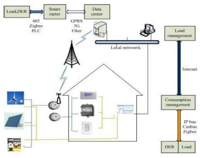
Figure 5. The communication grid in DSM framework
