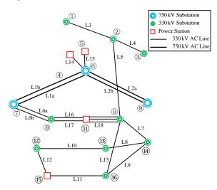
Figure 3. A section of the network wiring diagram of the power system
