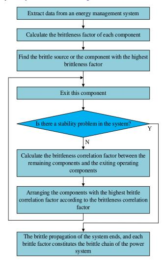
Figure 2. Method of determining the brittleness chain
