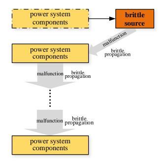
Figure 1. Brittleness propagation principle
