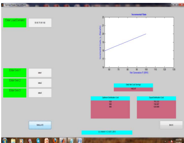
Figure 6. Sample screen for the lagrangian Optimal/Equal distribution cost with output of simulation, daily cost saving and incremental cost plot/data
