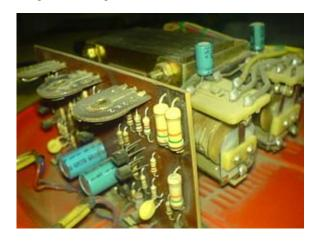
Figure 3.2. a voltage stabilizer using electromechanical relays for switching
