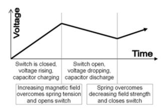
Figure 3.3. Graph of voltage output on a time scale
