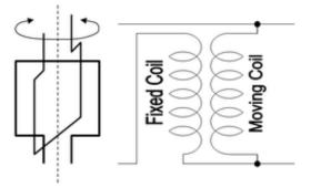
Figure 3.4. Basic design principle and circuit diagram for the rotatingcoil AC voltage regulator
