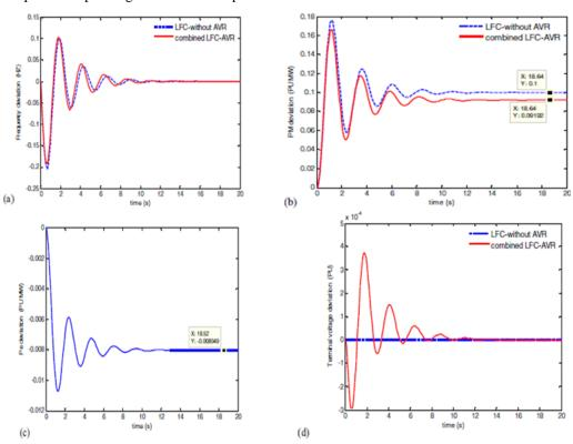
Figure 6.0. (a) Frequency deviation (rad/s), (b) Turbine output power (pu MW), (c)Terminal voltage deviation (pu), (d) Internal electrical power deviation (pu) (Results for this operating condition: P=0.9 pu, Q=0.5 pu, Vt=1 pu)
