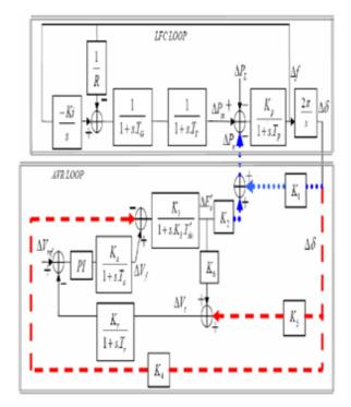
Figure 5.1. proposed combined model for LFC AVR loops
