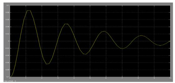
Figure 6.4. PE DEVIATION WITHOUT AVR
