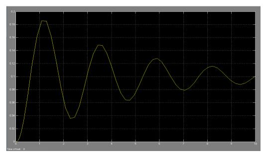
Figure 6.5. TERMINAL VOLTAGE DEVIATION WITHOUT AVR
