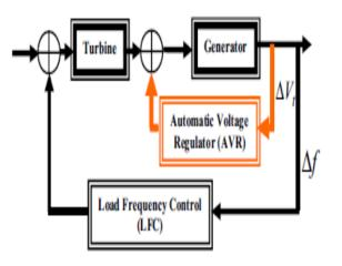
Figure 1.1. Automatic generation control with LFC and AVR loops
