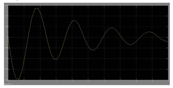
Figure 6.2. FREQUENCY DEVIATION WITHOUT AVR
