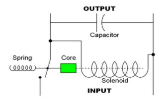
Figure 3.1. Circuit design for a simple electromechanical voltage regulator
