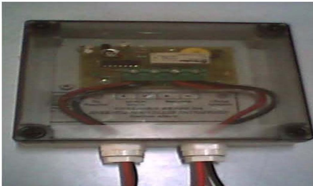
Figure 8. b: The used regulators for Batteries
