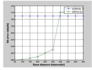
Figure 5. Bit error rate comparison of EEBPCB and EBPCB with distance form base station
