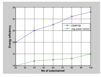
Figure 2. Energy efficiency comparison for EEBPCB and average power control algorithm for different no of subchannels
