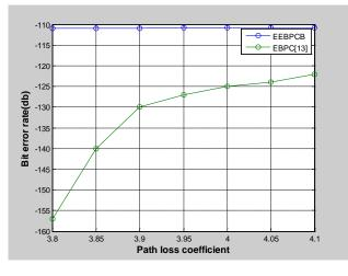
Figure 4. Bit error rate comparison of EEBPCB and EBPCB as a function of different path loss coefficients
