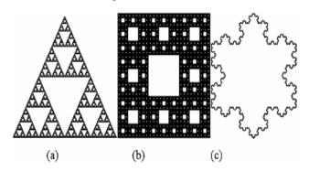
Figure 1. A typical view of common fractal antenna geometry (a) Sierpinski Gasket (b) Sierpinski Carpet (c) Koch Snowflake
