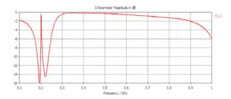
Figure 4.1. Variation of reflection coefficient (s11) with frequency
