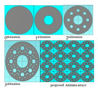
Figure 3.1. Multiple iterations of sierpinski fractal antenna using circular shapes & proposed 16 element Antenna arrays
