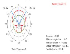
Figure 4.6. Polar radiation pattern (Gain) at fr=0.222 GHz
