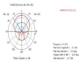
Figure 4.5. Polar radiation pattern (Directivity) at  $f_r$ =0.222 GHz
