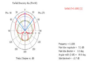
Figure 4.3. Polar radiation pattern (Directivity) at fr=0.1936 GHz
