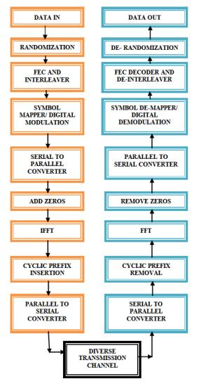
Figure 2. Simulation model of WiMAX-PHY layer
