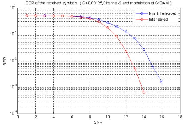
Figure 13. Effect of Block interleaver in 64-QAM on Channel-2
