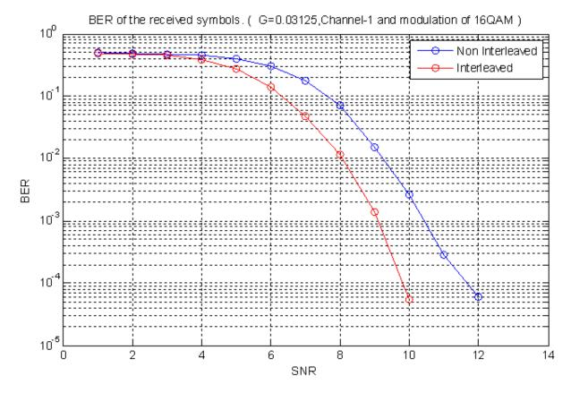
Figure 10. Effect of Block interleaver in 16-QAM on Channel-1
