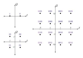
Figure 5. BPSK, 4-QAM, and 16-QAM constellation diagrams [10]
