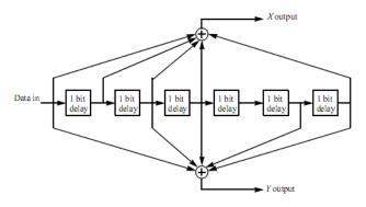
**Figure 4.** Convolutional Encoder of mother code rate  $\frac{1}{2}$  [3]
