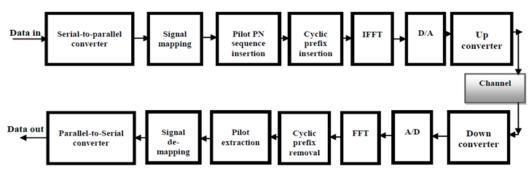
Figure 1. Block diagram of an OFDM Transceiver
