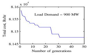
Figure 4. Convergence characteristics of proposed method with  $P_D$  = 900 MW (EED problem)
