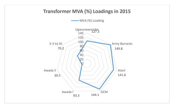
Figure 6. MVA Loading of transformers at the sampled Injection substations in Onitsha distribution network in 2015
