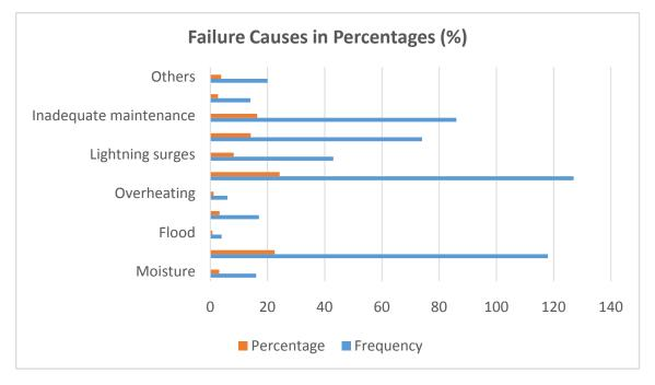
Figure 5. Classification of failure cause by percentage during 2011-2015
