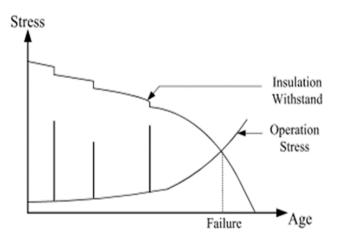
Figure 1. Transformer failure illustration [18]
