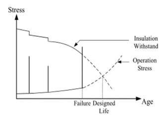
Figure 2. Transformer failure before expiration of designed life span [18]
