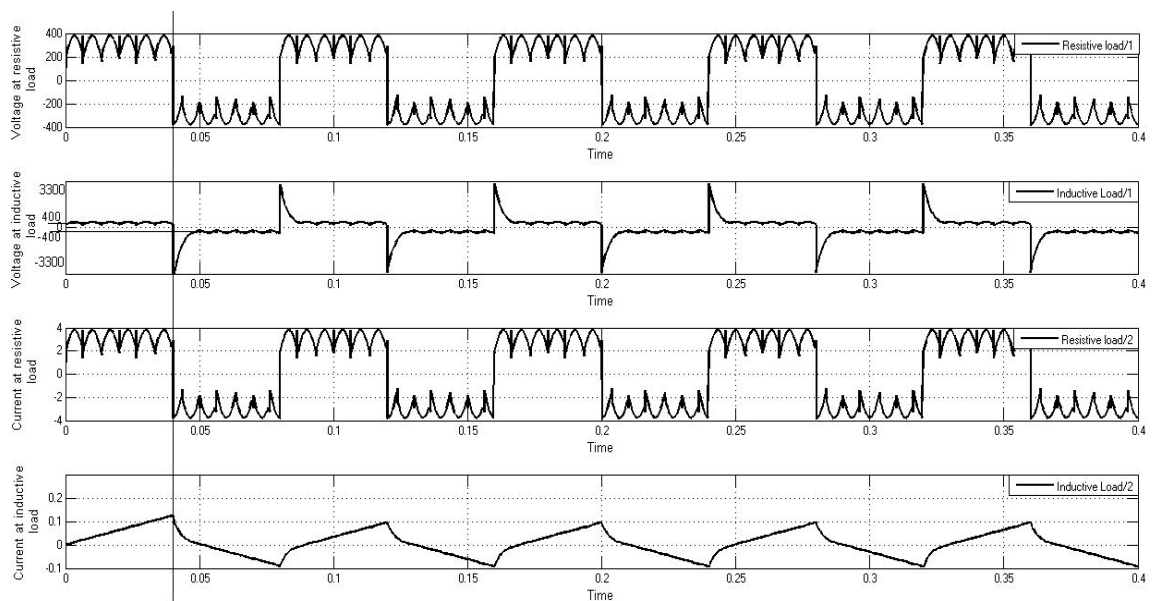
Figure 11. Resistive and Inductive Load Effect of 3Φ to 1Φ Cycloconverter
