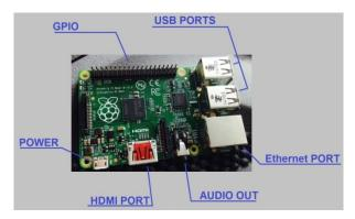
Figure 12. Raspberry PI3 component
