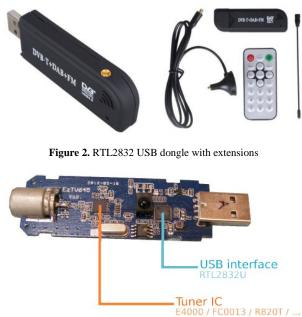
Figure 3. RTL2832 USB dongle internal design
