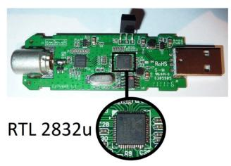
Figure 6. RTL2832U chip
