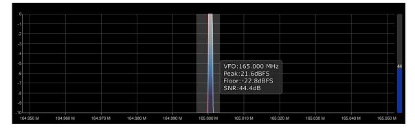
Figure 2. Signal strength when the transmitter facing the opposite side of the parasitic element that is shorted by inductor
