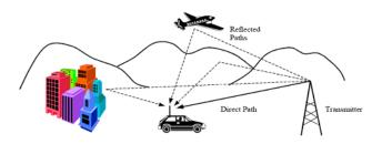
Figure 1. Effect of multipath on mobile receiver
