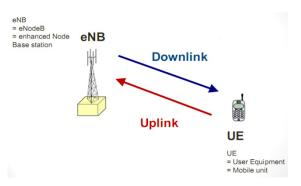
Figure 2. The uplink and downlink nomenclature for LTE networks
