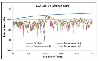
Figure 3. Return loss measurements of CCA cable 2
