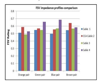
Figure 13. FSV impedance profile comparison between measurements A and C
