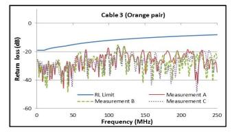
Figure 4. Return loss measurements of cable 3
