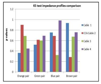
Figure 15. KS test p values chart for impedance profile comparison between measurements A and C
