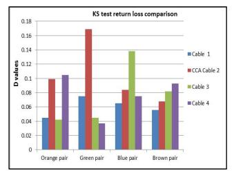
Figure 7. KS test D values chart for return loss comparison between measurements A and C
