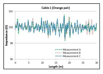
Figure 9. Impedance profile measurements for cable 1
