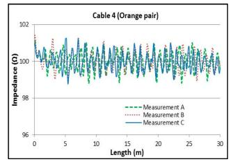
Figure 12. Impedance profile measurements for cable 4
