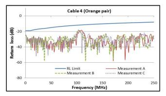
Figure 5. Return loss measurements of cable 4
