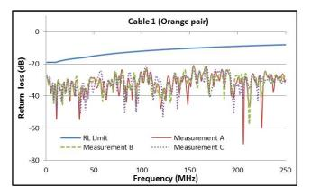
Figure 2. Return loss measurements of cable 1
