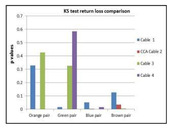
Figure 8. KS test p values chart for return loss comparison between measurements A and C
