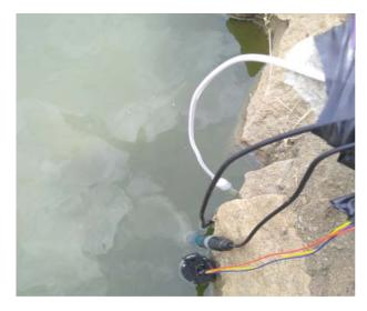
Figure 5. Sensor Probes deployed in the pond
