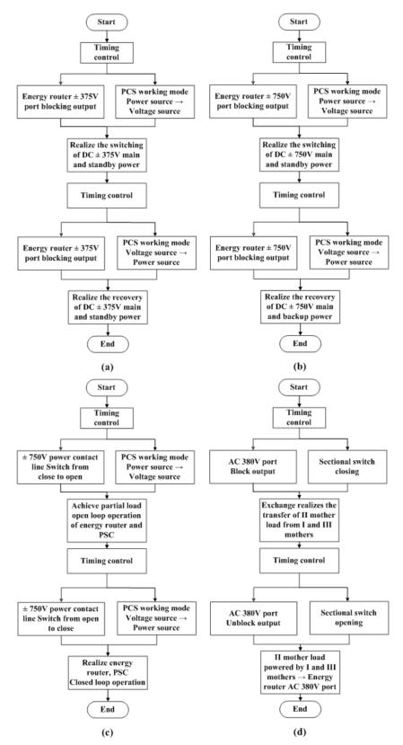
Figure 5. Flow chart of coordinated control method when operating mode is switched
