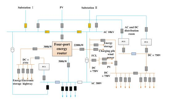
Figure 4. AC/DC distribution network system model
