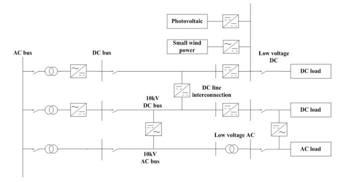
Figure 1. Typical Network Form of Medium Voltage AC/DC Distribution Network with DC Network
