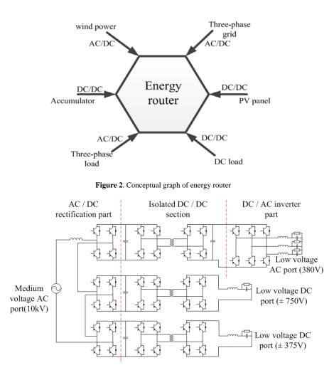
Figure 3. Topology of four-port energy router
