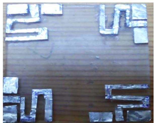
Figure 3. (a) 4-element MIMO antenna system on a glass window
